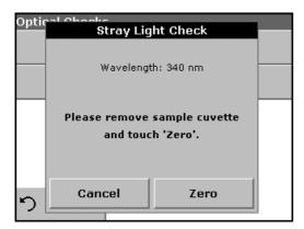
The Stray Light test is used to measure the stray light in the instrument at 340 nm.
